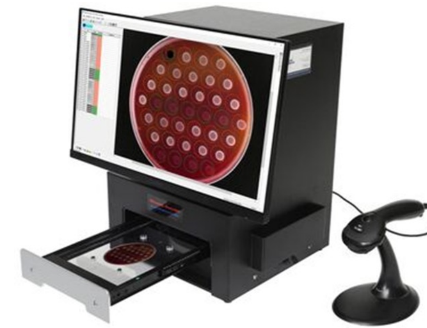
Figure 5. BIOMIC V3 automated agar dilution plate reader. Plates are placed in the imaging drawer with a custom 6x6 square plate holder and read with the BIOMIC V3 software. Image from Giles Scientific Inc.
