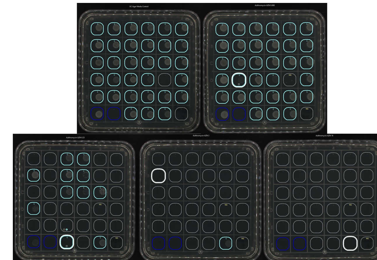
Figure 6. Automated reading. Images taken by the BIOMIC V3 during automated reading of agar dilution plates. The color bordering an isolate indicate growth (cyan), no growth (grey), indeterminate growth (yellow), or isolates not being evaluated (blue).
